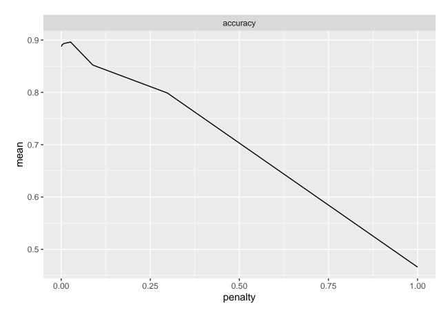
To tune lambda, I have used accuracy as the metric which is basically the proportion predicted correctly. This is a good metric in this case since our data is pretty balanced. As it can be seen by the confusion matrix that the numbers are around the same. By the graph above, the optimal lambda that will have great accuracy seems to be around 0.02 and if we keep increasing lambda, our accuracy will greatly decrease linearly.
